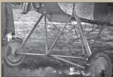
Undercarriage detail from Fokker E.III wn364 (possibly 111/15) showing strut fairings and rigging details.
