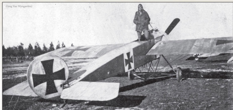
This unidentified late production Fokker E.III features late style eisernkreuz and a dark camouflage colour applied unevenly to the top of the wings. The top of the fuselage and elevator appear to have been doped or painted a very light colour, possibly the same colour that was previously applied to the outer sections of the wings.
